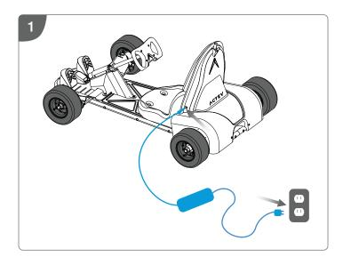
Plug the charger into the wall outlet and plug the other end into the charger jack on the left side of the Arrow.
