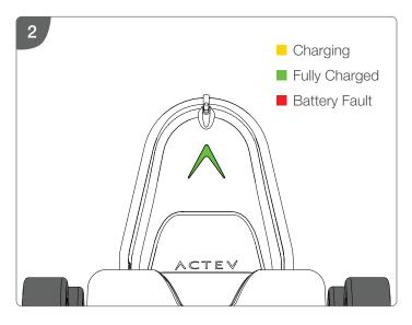
The rear light will turn yellow to indicate charging. When fully charged, the light will turn green.
